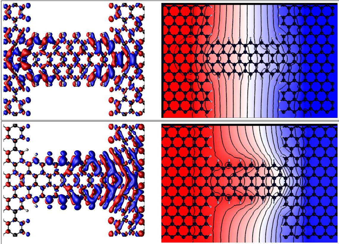
Figure 1: Charge redistribution with respect to  $V_{\text{bias}} = 0$  V (left figures) and potential drop (right figures) of the nano-constriction device upon application of a  $V_{\text{bias}} = 0.5$  V. Top panel shows the case for no doping  $n = 0e$  and bottom panel show  $n = -0.5e$  ( $p$ -type).
